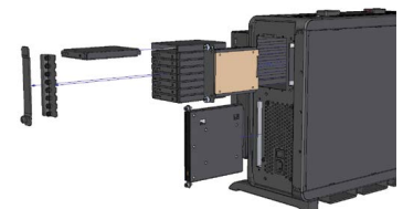
Mass data storage supports five removable 2.5" data disks or four 3.5" data disks and a pair of removable system disks. The optical drive is also quick swap as shown below.
