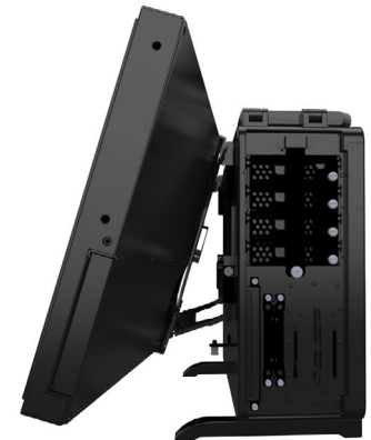
Side view showing MaxPac-8212ML3 display tilt-up adjustment as well as the hard drive and optical disk magazines
