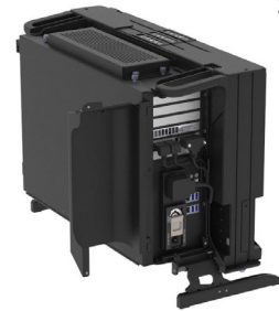
Side doors cover I/O without restricting airflow
